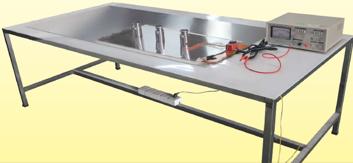
Device for measuring the insulation resistance. The measured values are always greater than 0.1Gohm
